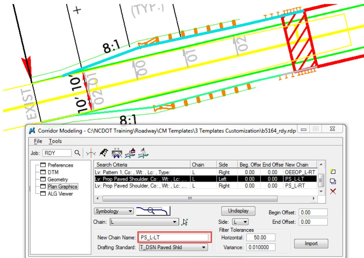
Note that the **Drafting Standard** selection only applies to the targeted style constraints. Usually this is how the paved shoulder location is defined. For purpose of this demo, Point Controls, along with the New Chain Name, will be used instead.
