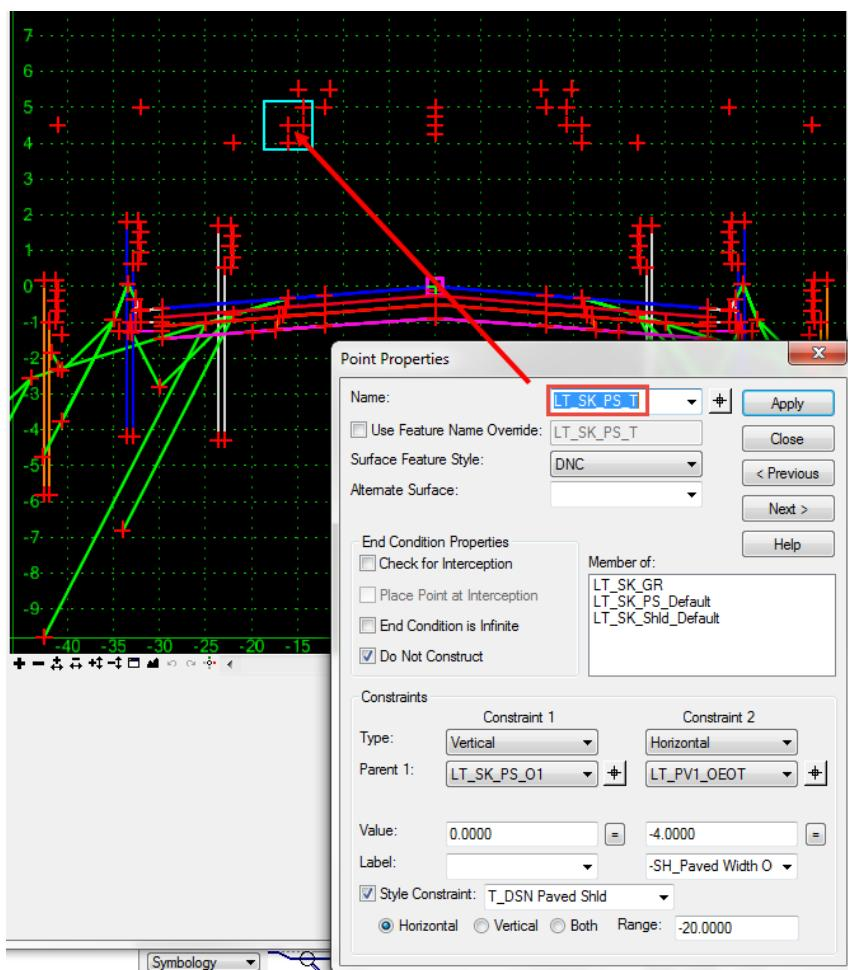
In Point Controls select this template point and move it horizontally to the location of the **PS\_L-LT** chain name.
