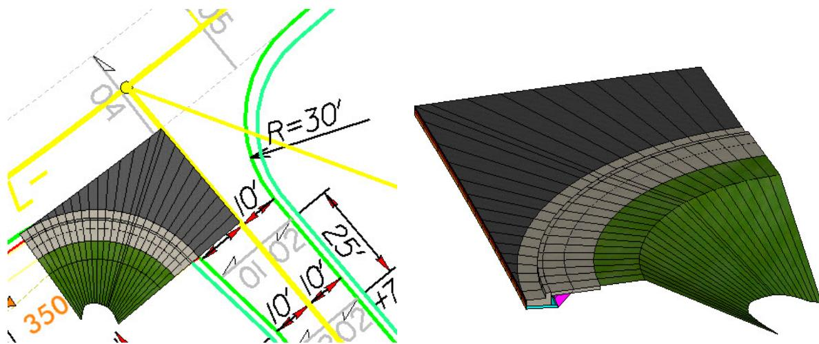
Similar to Corridor Points, the 3D features generated when the DTM was created can be used as Point Controls. The following is from the Hydro Ditch Delta Training. The objective was to move the template shoulder point **RT\_GS\_OS\_CTL** to the horizontal and vertical location of the same roadway feature name **RT\_GS\_OS\_CTL** (shoulder point).
