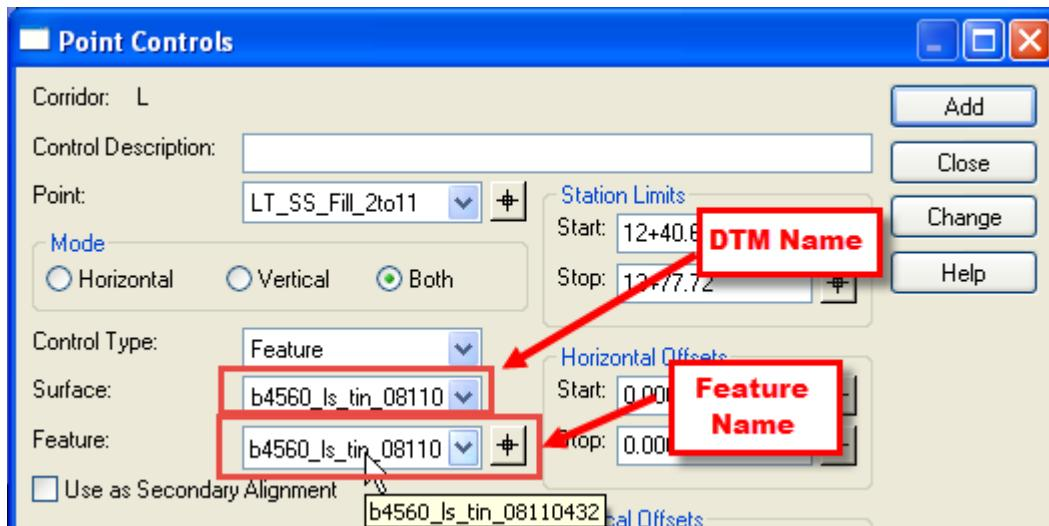
With this approach, Point Controls can be used to tie the fill slope to an existing feature (breakline in the DTM).
