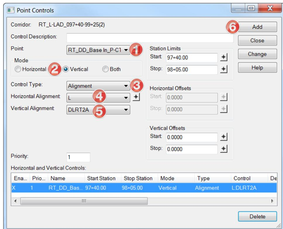
For projects without ditch grades stored in the GPK/Geometry, use the **Elevation and Grade** (with station ranges) option as the control type.
